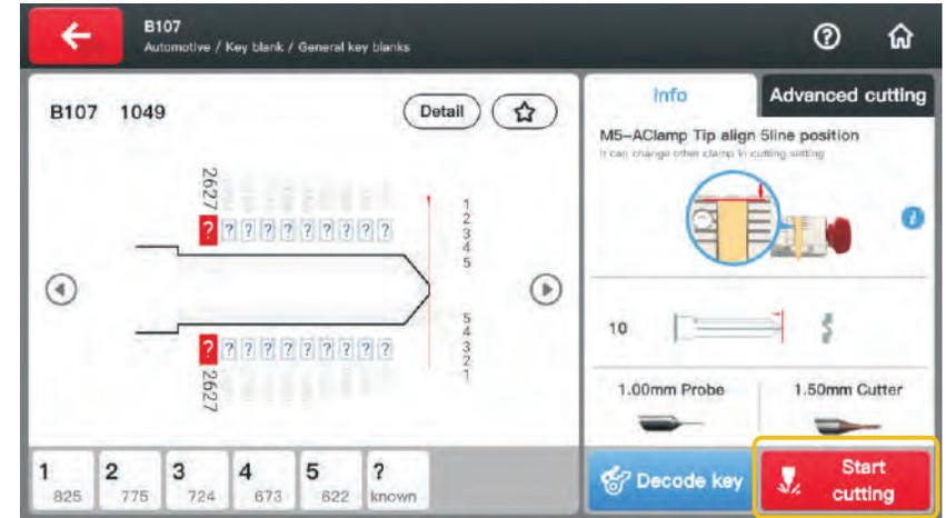
4) Install the key blank according to the diagram on the right, enter the key code and click "Start cutting".
